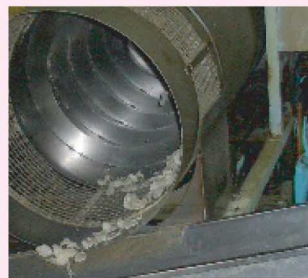
9. after oil is drained by a centrifuge, protruding portions are removed.
